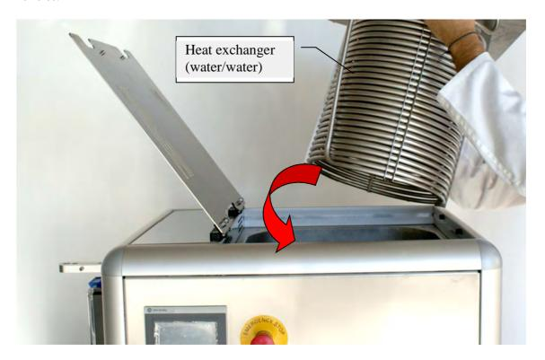
As can be seen, the heat exchanger has a water inlet and a water outlet, for the connection of a silicone pipe of 8x2.4 mm.
